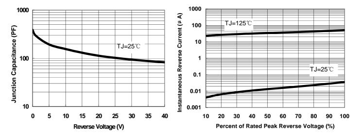
Fig.1-Typical Junction Capacitance
