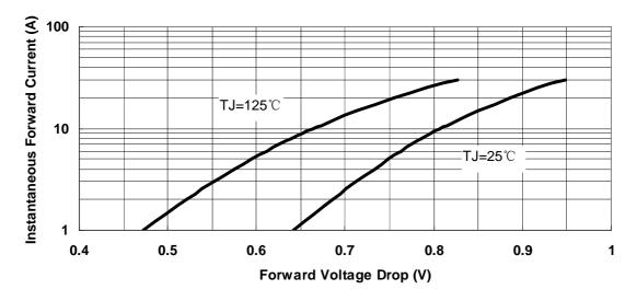
Fig.3-Typical Instantaneous Forward Voltage Characteristics
